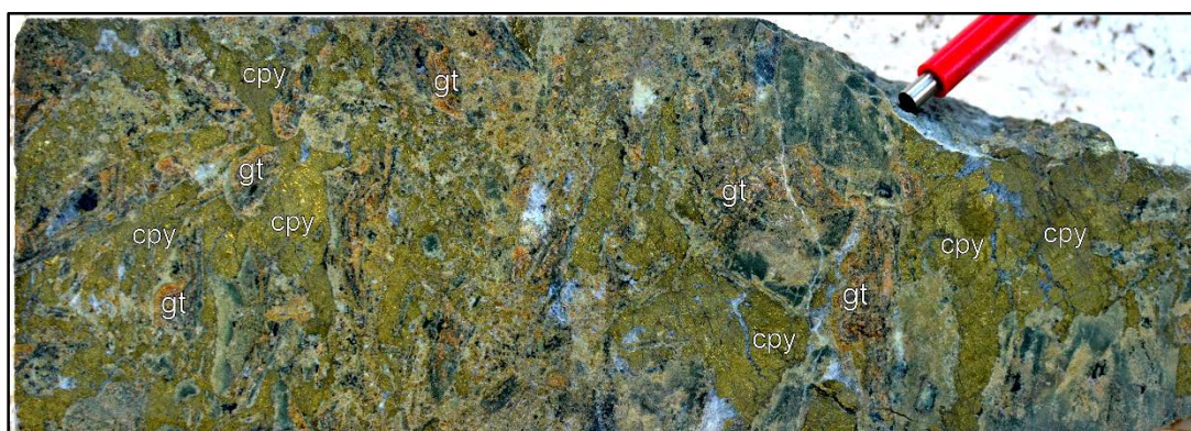
Figure 13: Garnet (gt) skarn with high-grade chalcopyrite (cpy) mineralisation and no magnetite. MDH-95, 122m.
