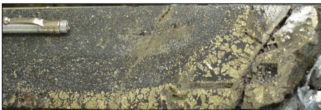
Figure 12. High-grade chalcopyrite in magnetite skarn, MDH-60, 212m.
