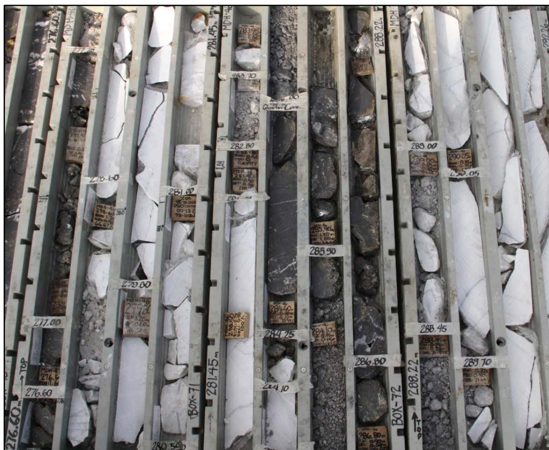
Figure 10: Massive magnetite skarn in sharp interfingering down-dip contact with white marble after limestone. MDH-46, 280 m.
