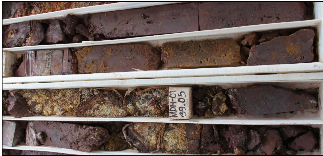
Figure 19: Oxidised hematitic mineralisation after massive magnetite skarn with intervals of deeply weathered calc-silicate hornfels or skarn. 63 mm HQ core, MDH-01.
