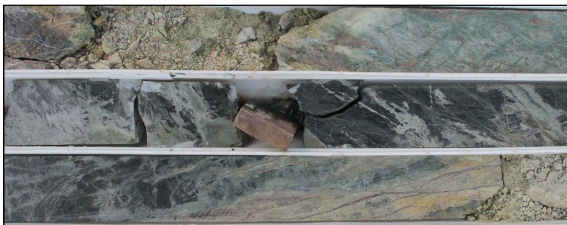
Figure 15: Hornfels after siltstone and calcareous siltstone overprinted by strongly retrogressed calc-silicate (pyroxene) skarn with zones of strong oxidation. MDH-35, 183m.
