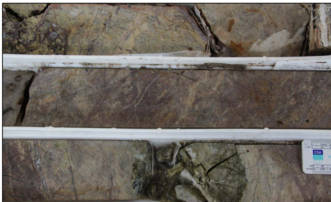
Figure 14: Massive garnet skarn strongly retrogressed to epidote, sericite and chlorite. MDH-09, 121 m. HQ core, 63mm diameter.
