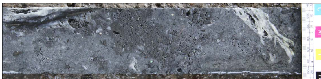
Figure 17: Vuggy silica-pyrite altered breccia with arsenopyrite. MDH-13, 128.6 m.
