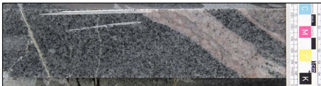
Figure 8: Quartz diorite with late quartz-feldspar veins and minor sericitic alteration around later thin quartz veins. MDH-24, 57 m.
