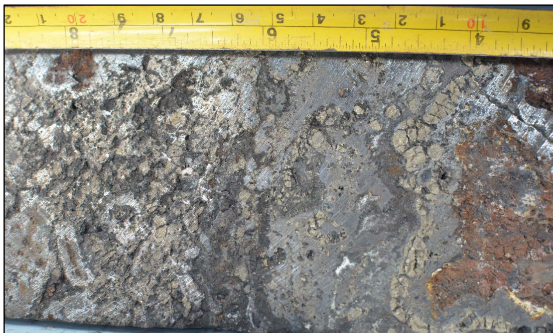
Figure 18: High-grade bornite associated with pyrite overprint of magnetite skarn. MDH-66, 79m.
