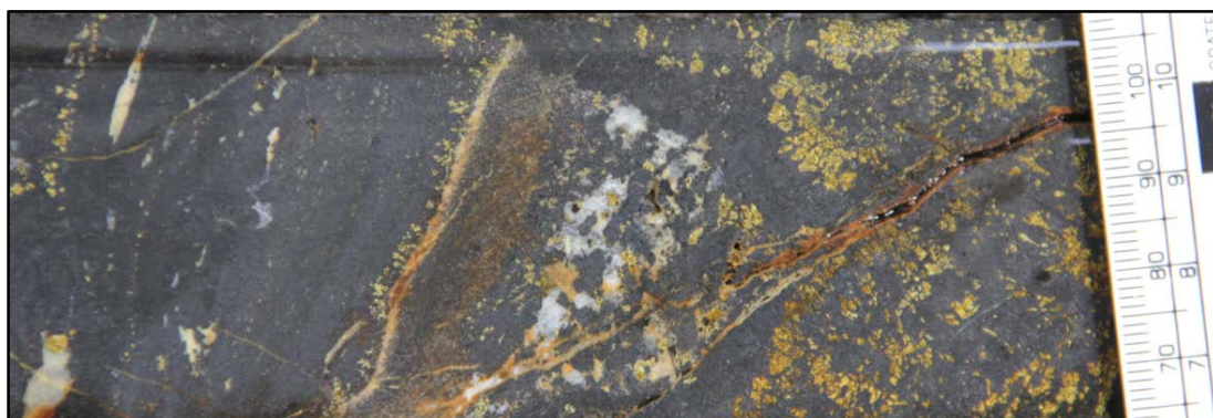
Figure 11: Crudely banded massive magnetite skarn with remnant calc-silicate band on left. High-grade magnetite-chalcopyrite mineralisation on right cuts earlier banded magnetite-chalcopyrite-calc-silicate with interstitial calcite in centre. MDH-016, 139.5 m.
