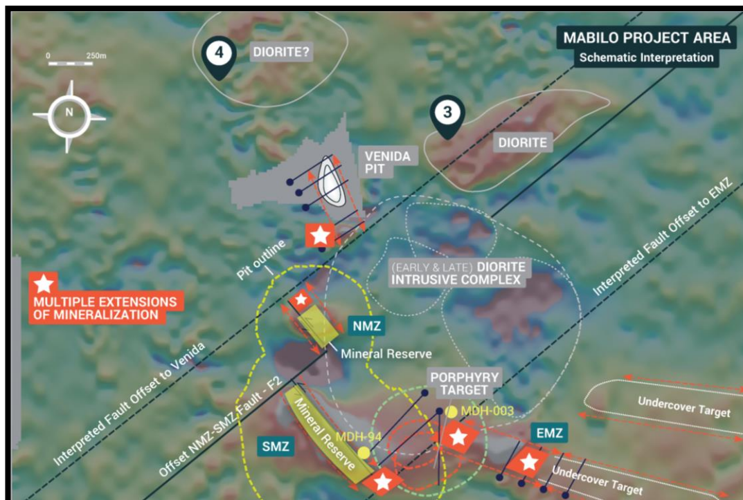
Figure 1 - RTP ground magnetic image with modelled South, North and East magnetic bodies, showing exploration upside targets.
